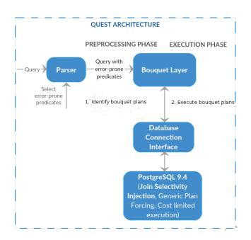
Figure 4.1: Modified QUEST Architecture
