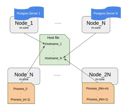
Figure 5.2: Parallel architecture for POSP Identification
