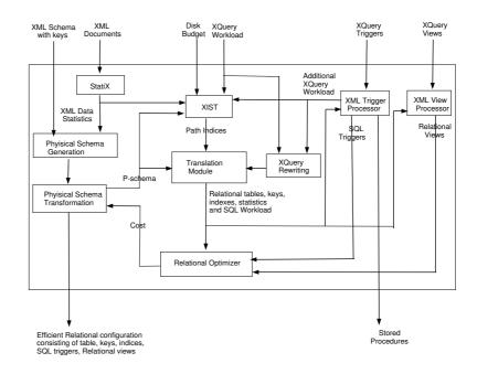
Figure 1.4: Architecture of the Elixir system
