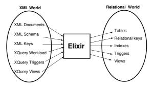
Figure 1.3: Our proposed XML-to-relational Mapping approach
