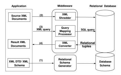
Figure 1.1: A typical system for storing XML using RDBMS
