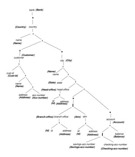
Figure 4.1: Schema tree for bank schema
